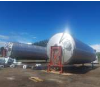
Glycerine tanks V=150 m3 - before insulation and insulated
