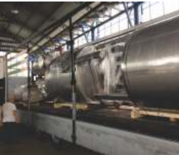
Sugar pulp heaters/mixers (Brittish sugar, United Kingdom)
