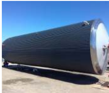
Glycerine tanks V=150 m3 - before insulation and insulated
