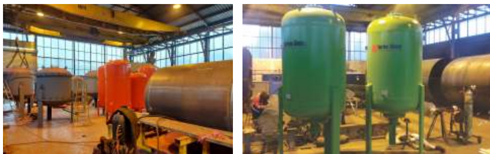
Pic2. Anti-surge membrane vessels of various sizes and nominal pressures up to 80bar
