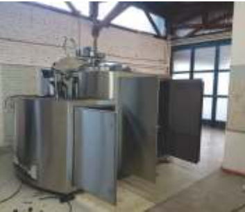
Shaving paste production reactors (Micra GmbH, Germany)
