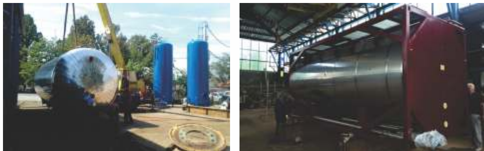
Pic1. Various vessels (2x15m 3 comp.air units, heating autoclave, LPG container tank) waiting for dispatch
